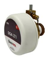
Qualitrol's DGA LT1 is a wireless, self-powered dissolved gas analyzer that monitors hydrogen, moisture, and temperature int he dielectric insulating oil at a breakthrough price. Installation takes minutes because there is no need to install power or communication cables.
